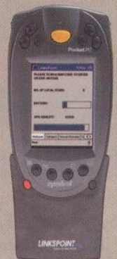
Symbol Technologies' PPT 2800 with LinksPoint GlobalPoint GPS and Field Data Collector software
